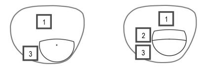
Figure 2: Structure of a bifocal lens (left) and a trifocal lens (right)
