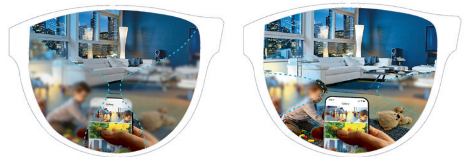
Figure 1-26: Restrictions in the fields of vision by the base curve effect (left), no restrictions (right)
